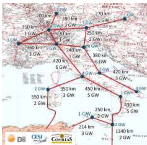
Figure 9 Grid reinforcement Central corridor Option II
