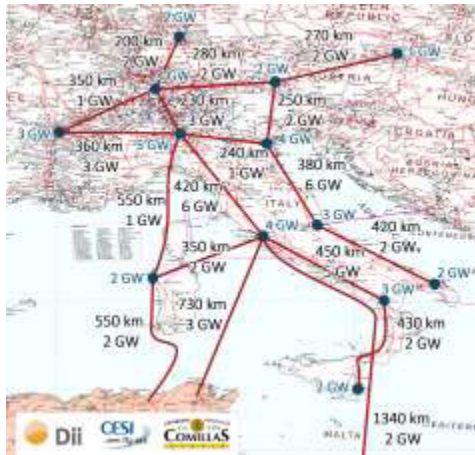
Figure 8 Grid reinforcement Central corridor Option I
