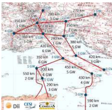
Figure 10 Grid reinforcement Central corridor Option III
