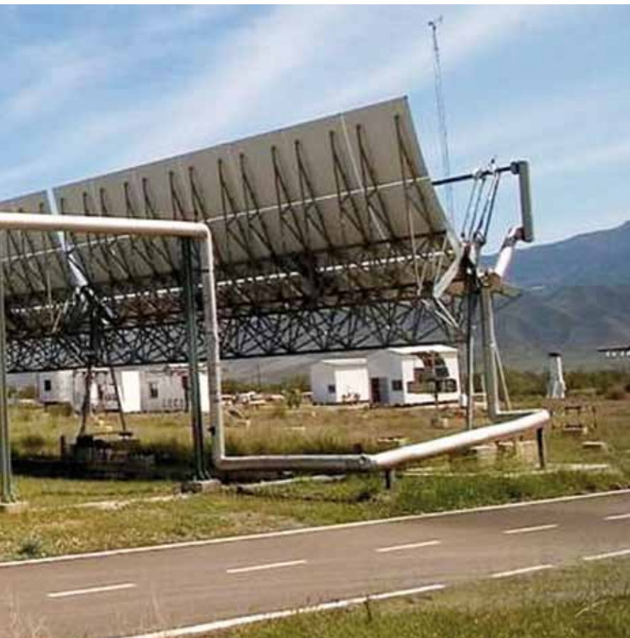
The PSA HTF test facility, which is used for evaluation of new components and parabolic trough designs (CIEMAT-PSA, Plataforma Solar de Almería)
