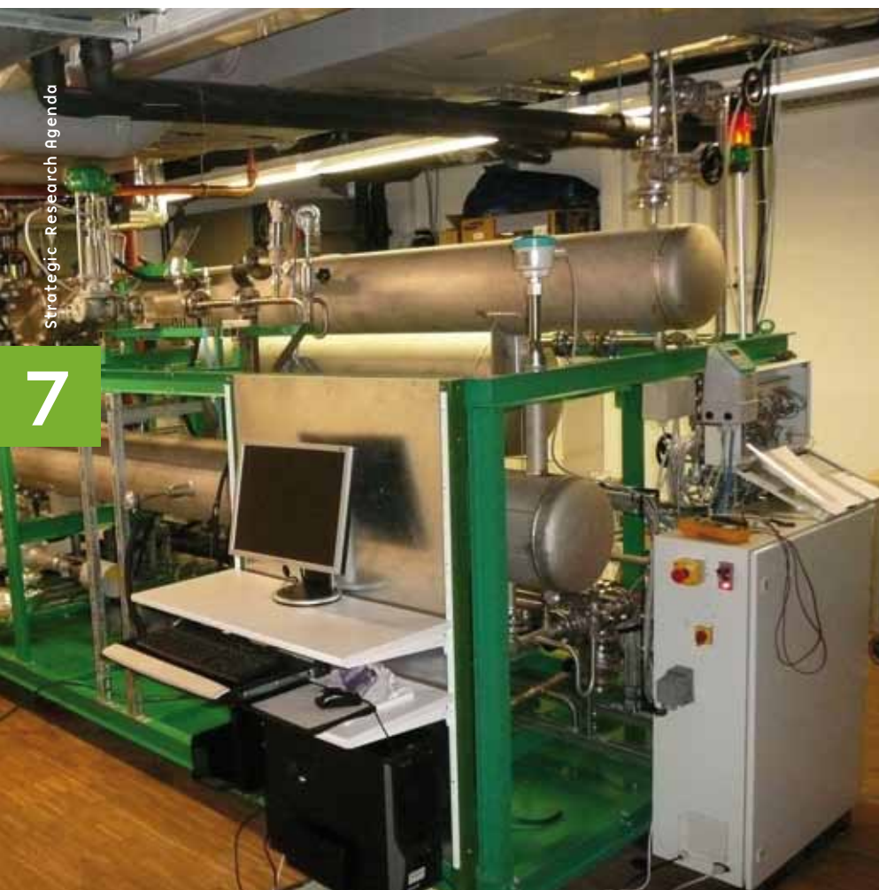
Laboratory at Fraunhofer ISE for testing the dynamical operation of high temperature storage systems and small steam heat engines for combined heat and power. The steam output of a solar field using concentrating collectors is simulated in real time by a gas heater with evaporator
